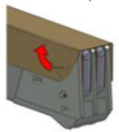
3. Remove the screws on the bottom side of the seal bar.
