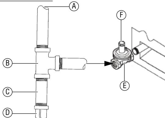
A To gas supply with the installation of B, C and D in a vertical orientation as shown to provide for debris capture.
