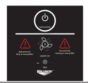
4. Press the LED switch to turn lights on or off.
