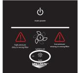
3. Press Main Power switch to exit LED setup mode. NOTICE: When the control is on and the function enabled, the switch and indicator will be visible.
