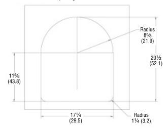
3. Measure and cut the opening for the control box.
