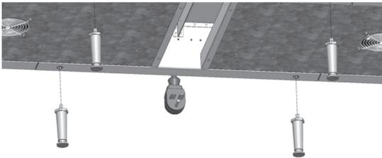
5. Install the load and unload trays to match the conveyor direction. The load tray slants toward the conveyor. The unload tray slants away from the conveyor.
