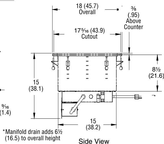
\*Manifold drain adds 6 1/2 (16.5) to overall height
