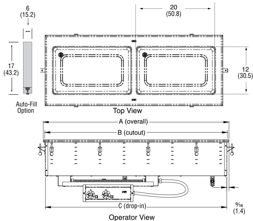
Controls must be mounted on the opposite side of the unit from the drain pipes to maintain proper orientation.
