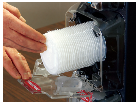
Illustration C Lids are uniform and evenly spaced right out of the sleeve. They will dispense very well.
